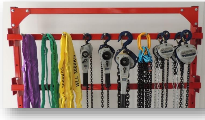
Example of a safe and tidy Lifting Gear storage
