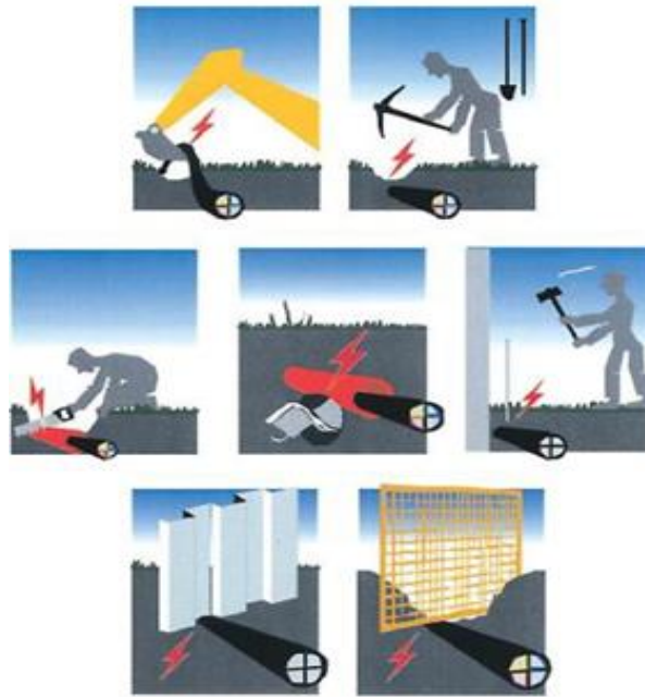
Examples of potential ways to impact underground services and endanger workers
